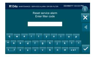
7) Type the filter code and press to delete the alarm. If the filter code is not available, call the Service Center
