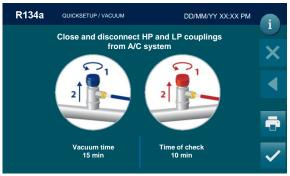
Close and disconnect HP and LP coupling from A/C system, then press
