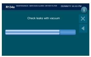
automatically the machine proceeds to the pressure control
