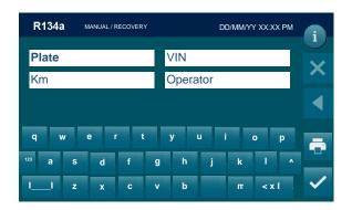
Type the plate of the car,VIN, Km, Operator and press to confirm.
