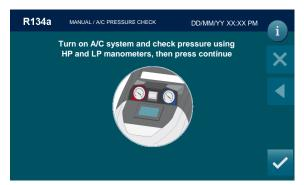
Turn on A/C system and check pressure using HP and LP manometers, then press :
