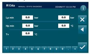
Type in, in order, the minimum value of low pressure, the maximum and minimum value of high pressure of the A/C system, and the temperature of the air at the outlet from the vents in the passenger compartment (use the thermometer supplied with the machine to measure).
