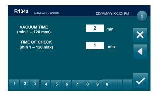
use the KEYPAD to insert the new value of the VACUUM TIME, press to confirm, to return back.
