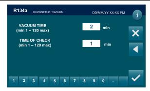
Use the KEYPAD to insert the value of the VACUUM TIME, press 🚩 to confirm
