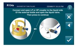
Connect and open LP or HP coupler to the liquid side of the external bottle and open the liquid valve. Then press to continue
