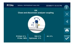
Close and disconnect analyzer coupling
