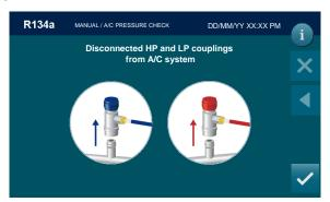
Disconnect coupling from A/C system, press to return to the MANUAL PROCEDURE MENU; A/C PRESSURES CHECK is now successfully complete
