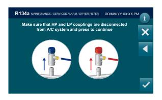
Make sure that HP and LP coupling are disconnected from A/C system or else and press  $\stackrel{\checkmark}{}$  , machine will check presence of refrigerant
