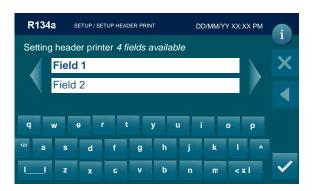
Use the keypad to modify the 4 lines, then press return to SETUP menu.
