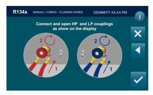
Connect the HP and LP couplers to the respective fitting on the machine, the press <a href="text-align: centinue">to to continue</a>:
