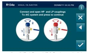
Connect and open the coupling (HP, LP, or HP/LP, depend of the previous choice) connected
