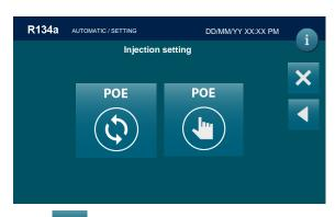
Select PAG/POE oil symbol AUTOMATIC injection for insert the gas quantities and reintegrate the same quantity of oil extracted during recovery. Select PAG/POE oil symbol
