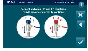
Connect and open the coupling (HP, LP, or HP/LP, depend of the previous choice) connected to the A/C system, then press , press to return back.
