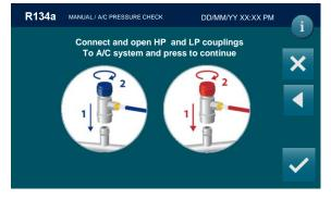
Connect and open the coupling connected to the A/C system, then press , press return back; the following screen is displayed:
