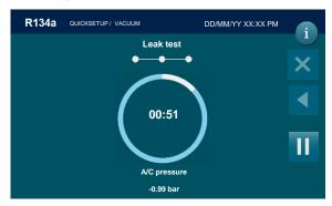
(WARNING! If vacuum time is lower than 15 minutes this test is not reliable). If leaks are found, the machine will stop automatically and display the A/C SYSTEM LEAKS alarm.
