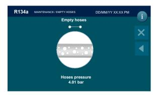
the machine will recover all the refrigerant into the service hoses; then the machine will sound and alarm and the following screen will be displayed:
