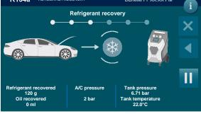
During the recovery phase, the machine displays the quantity of refrigerant recovered, in grams. Upon completion of recovery, the machine will stop and discharge, while automatically displaying the used oil extracted from the A/C system during the recovery phase. The oil discharge operation lasts 4 minutes.
