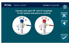
Connect and open the coupling connected to the A/C system, then press to start the
