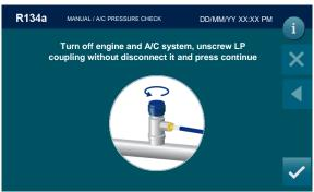
Turn off engine and A/C system, unscrew LP coupling without disconnect it, then press ✓:
