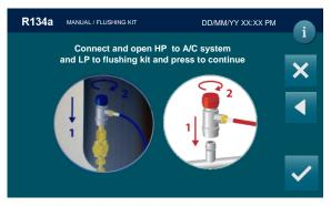
Connect and open HP to A/C system and LP to flushing kit and press to continue:
