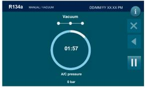
When time of check is reached, the machine will test for leaks in the A/C system:
