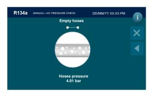
The machine will recover the residual refrigerant into the service hoses, then the following screen will be displayed:
