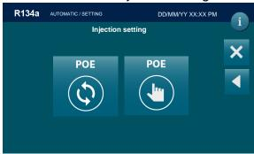
Select PAG/POE oil symbol AUTOMATIC injection for insert the gas quantities and reintegrate the same quantity of oil extracted during recovery. Select PAG/POE oil symbol
