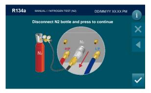
Disconnect coupling, then press the following screen will be displayed:
