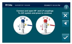
Connect and open the coupling connected to the A/C system, then press to start the vacuum phase
