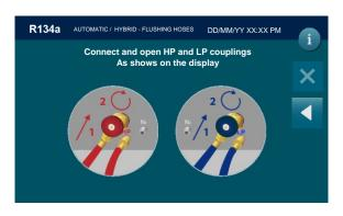
If HYBRID VEHICLE is selected the machine will perform FLUSHING HOSES
