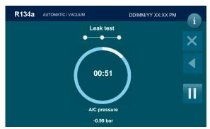
(WARNING! If vacuum time < 15 minutes this test is not reliable). If leaks are found, the machine will stop automatically and display the A/C SYSTEM LEAKS alarm.
