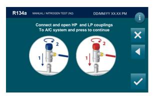
Connect and open HP and LP coupling to A/C system, then press OK to continue; the following screen will be displayed:
