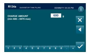
Use the touchscreen keys 0 to 9 to type the quantity (in grams) of refrigerant to be charged into the tank, then press
