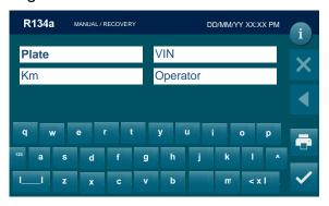
Type the plate of the car, VIN, Km, Operator and press to confirm. BACK to return back.
