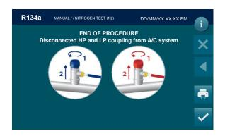
Unscrew and disconnect HP and LP coupling from A/C system end press to complete the N2 TEST.
