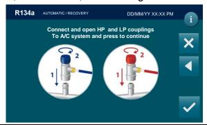
Connect and open the coupling to the A/C system, then press , press to return back. the following screen will be displayed:
