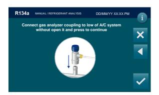
Connect gas analyzer coupling to low of A/C system without open it and press to continue
