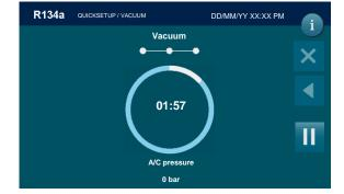
When time of check is reached, the machine will test for leaks in the A/C system:
